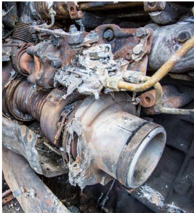
Figure 3 - A turbocharger after an engine bay mechanical fire.
