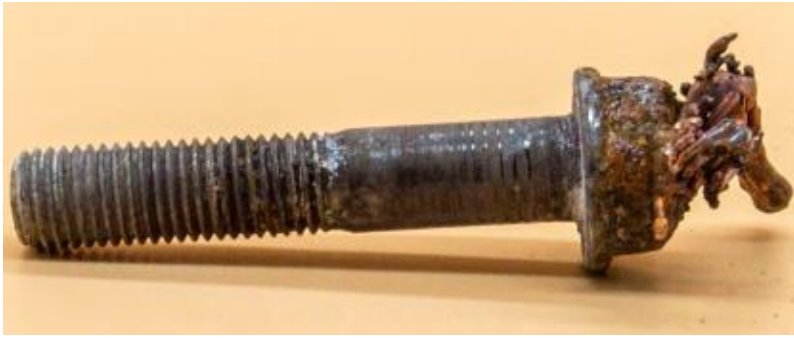
Figure 2 - A bolt that had rubbed through a power cable with the copper cable still welded to the head.
